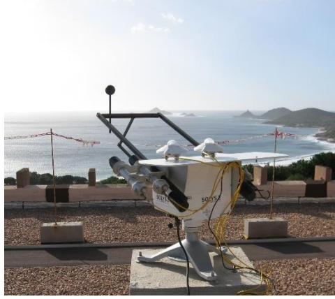
Figure 1.3.20. Pyrheliometer (beam radiation), pyranometer (global radiation) and pyranometer with shading black ball (for sky diffuse radiation).
