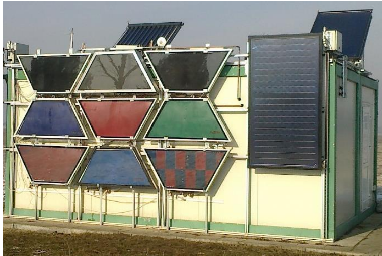
Figure. 2.2 Outdoor testing rig with flexible interconnection of the novel trapeze solar-thermal flat plate collectors
